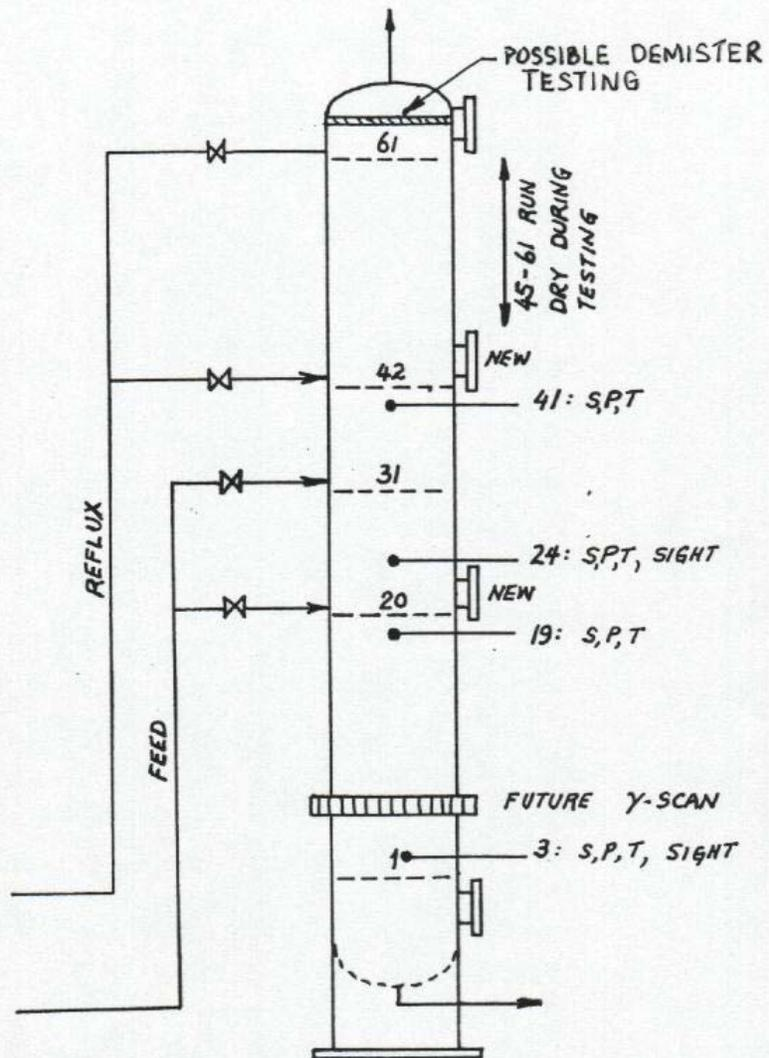
Figure 5 Detail of Column Revamp Showing Alternate Feed and Reflux Points, Positions of Sample Points (S), Pressure (P) and Temperature (T) Taps, Sight Glass Locations, and Position of Future One-Tray Detailed Gamma Scan
