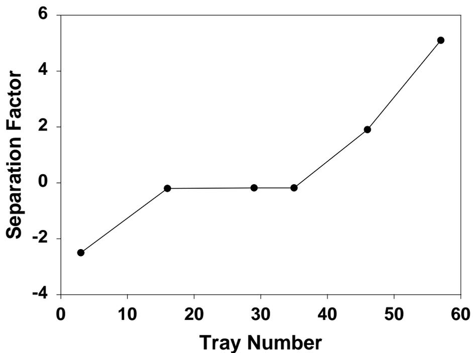
Figure 4 Separation Factor vs Tray Number From Bottom Showing Ineffectiveness of Middle 20 Trays (Pinch)
