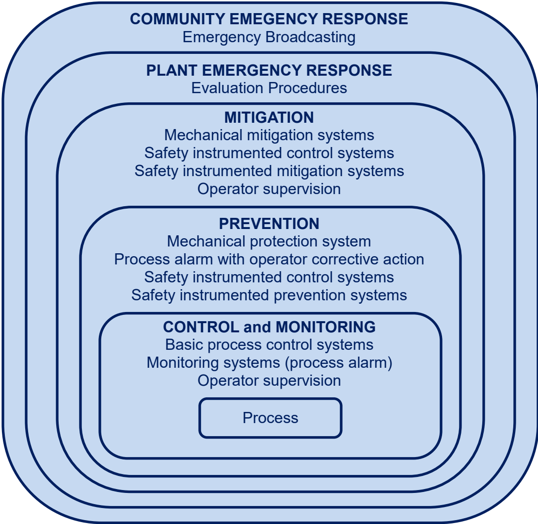
Figure 3: Typical protection layers in hazardous industrial installation
