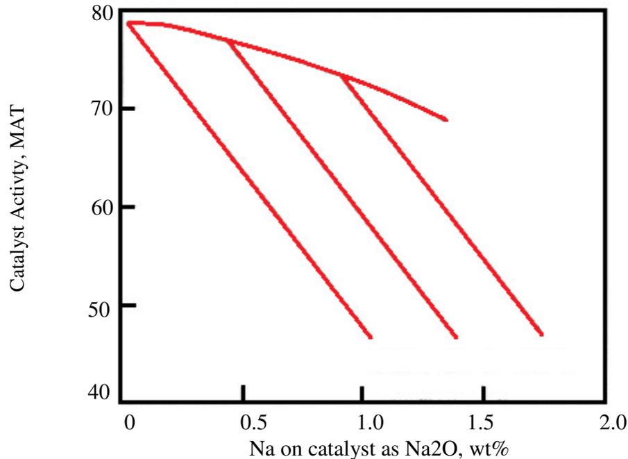
Figure 2: Catalysts activity loss from sodium contamination
