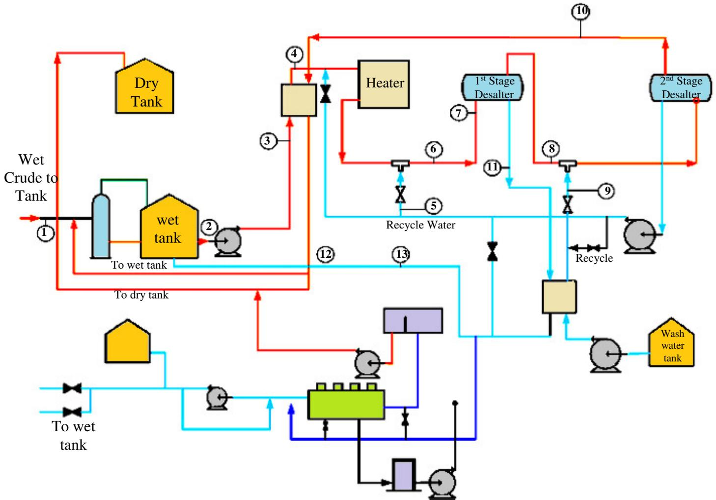
Figure 3: Schematic of crude oil desalting (7)
