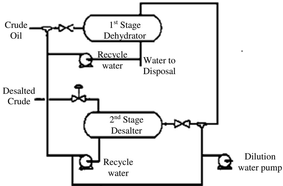
Figure 7: Two Stage Desalting with Recycle and Internal Recycle (9)
