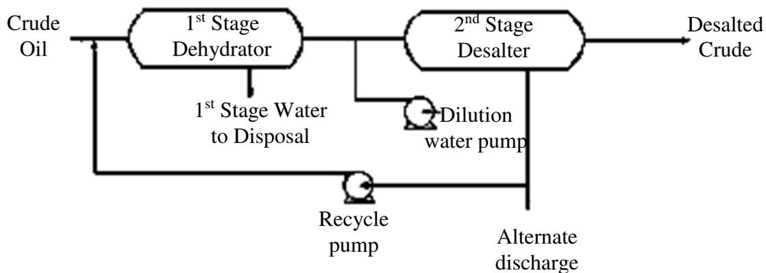
Figure 6: Two Stage Desalting with Recycle (9)
