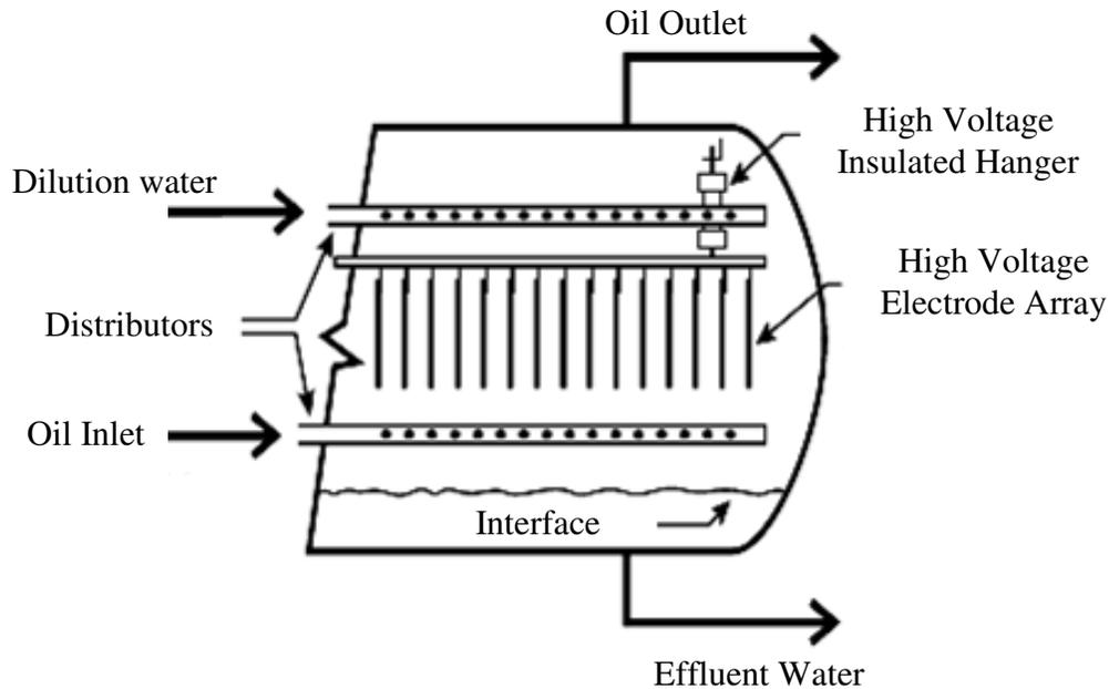
Figure 8: The Electrostatic Desalter System
