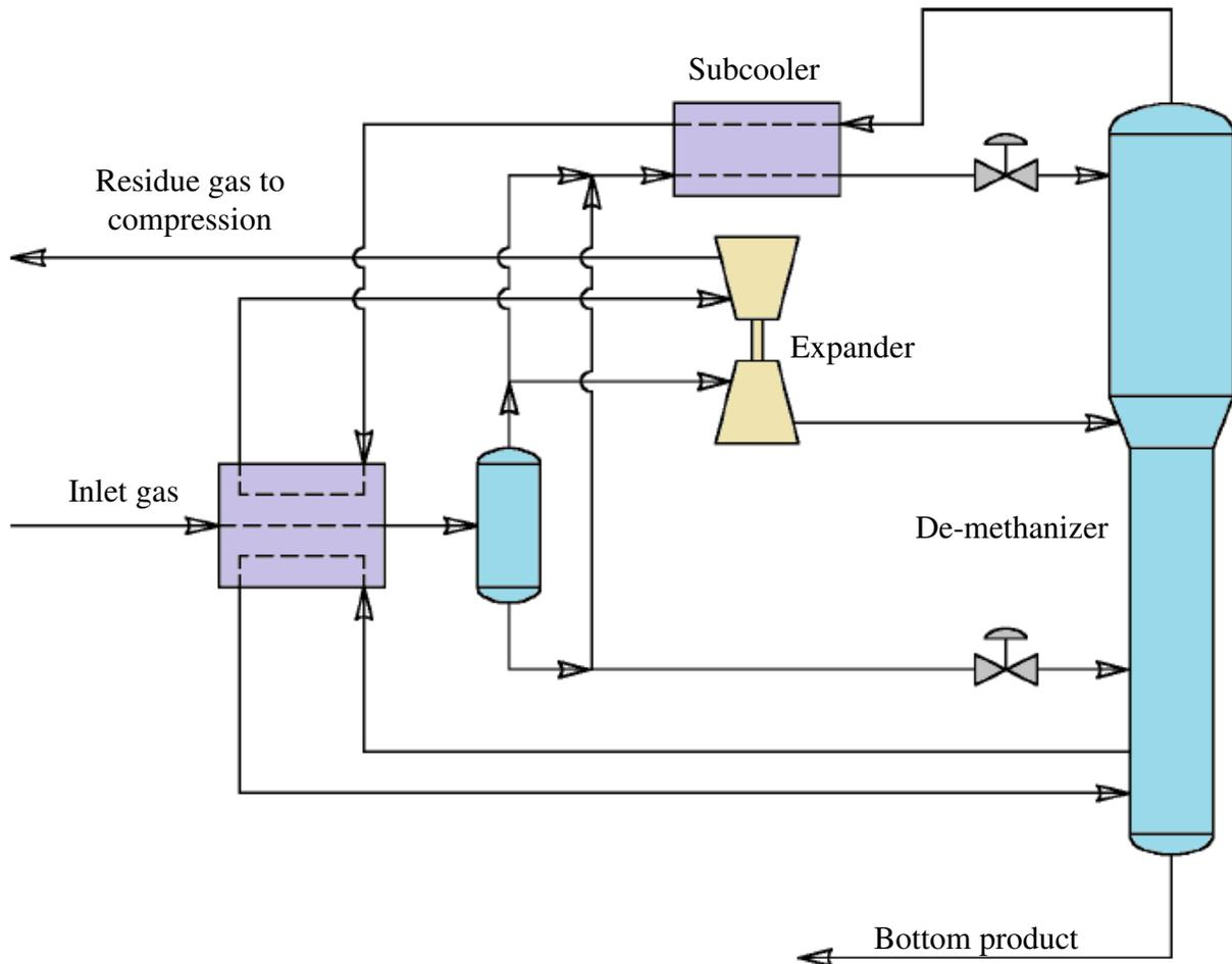
Figure 3: Schematic of GPC (gas subcooled process)
