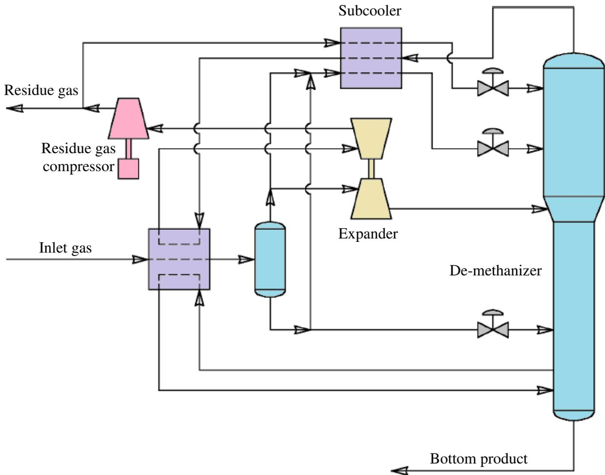
Figure 4: Schematic of residue split-vapor process
