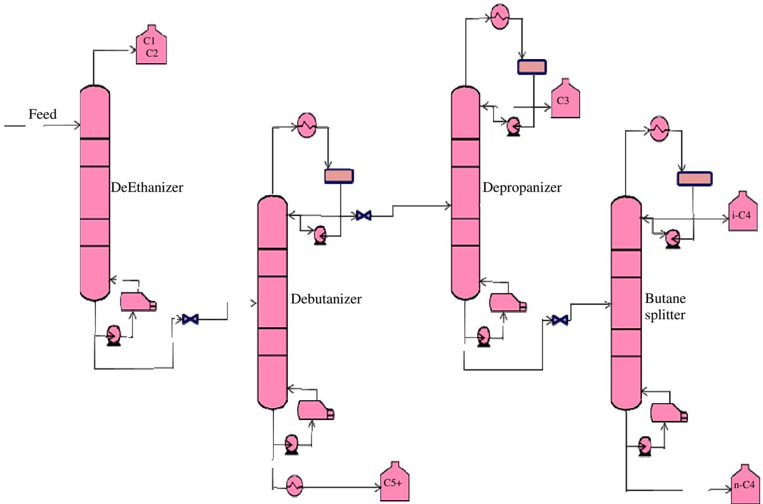
Figure 1: Process flow diagram of LPG unit
